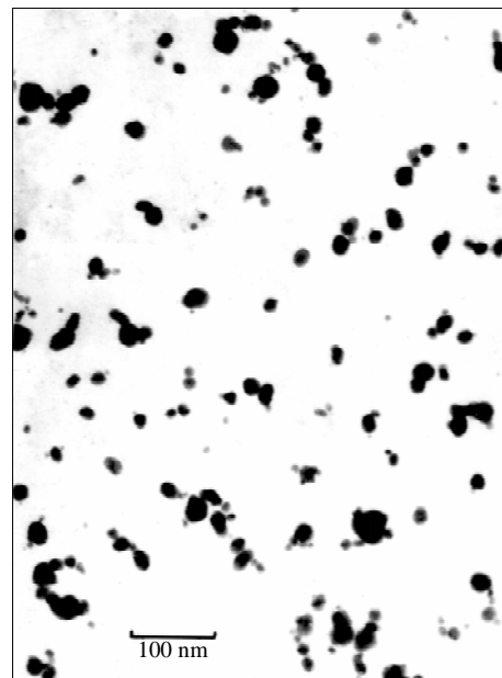
Figure 4 Photomicrograph of silver particles in an Ag–DMAEMA organic dispersion freshly prepared by the cryochemical synthesis.
